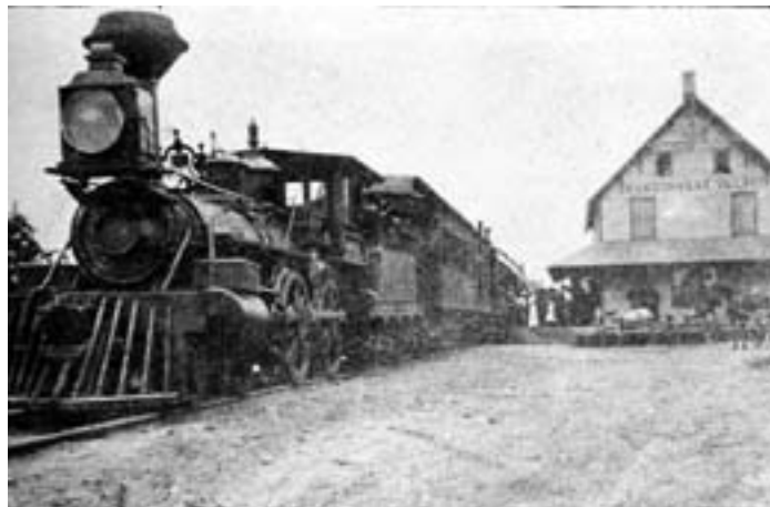
Arrival of the Orford Mountain Railway train in Mansonville Village Station around 1907. The engine burnt wood, not coal, and the large funnel shape chimney had a screen on top to prevent sparks from lighting fire along the tracks.
